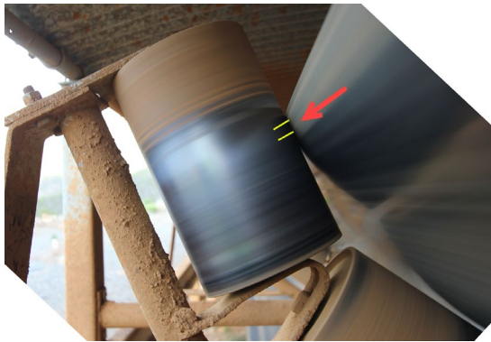
Fig. 16.1: Carcass too rigid for a deep trough.
