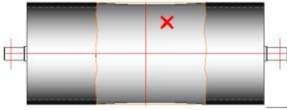
Figure 6.2 : Concave profile by wear (belt instability)
