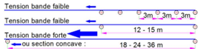
Figure 9: 3 m : non-compliant ; 12m : compliant
